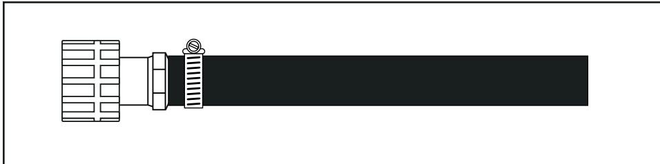
Figure 2: Poly-Pipe connected to Poly Adapter with Gear Clamp
